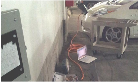
FIGURE 15. Experiment setup of changing pilot signal
