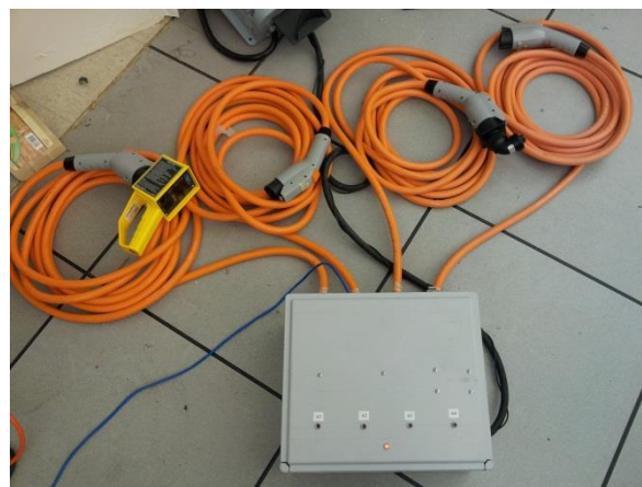
FIGURE 4. Realization of 4 channel charging station.
